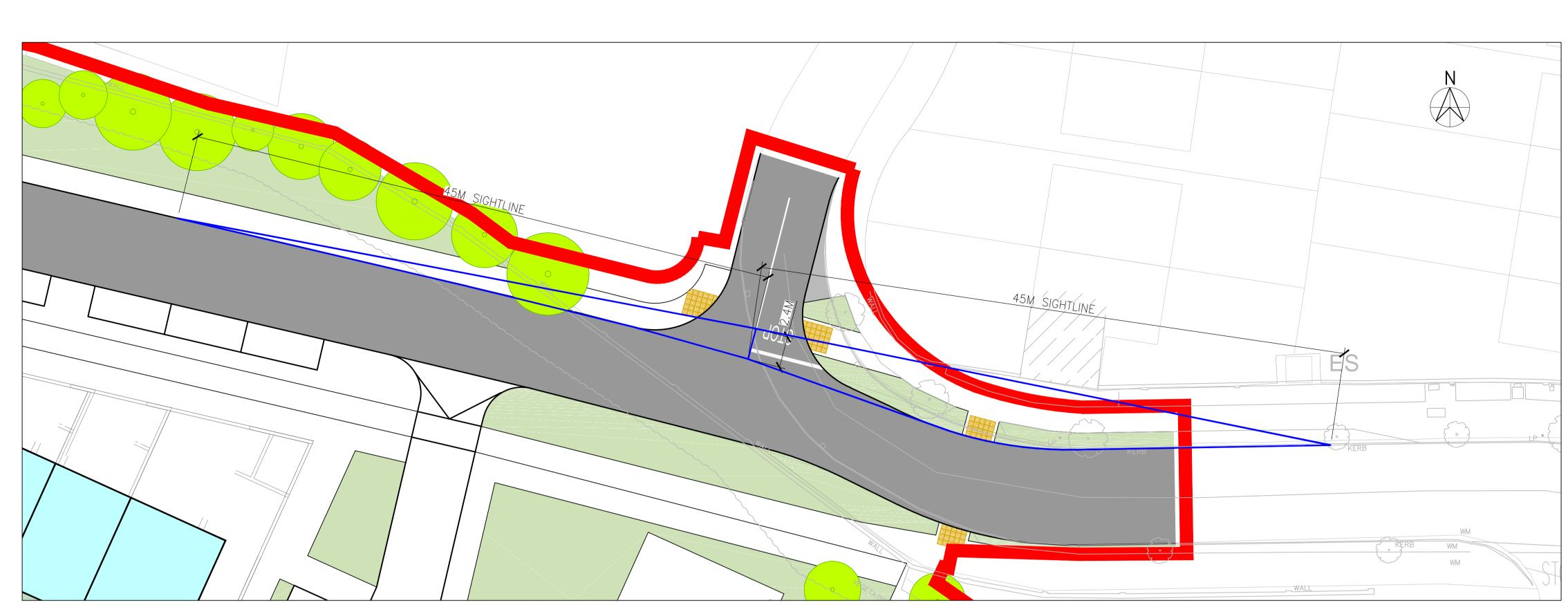
SIGHTLINE NO.1 FOR PROPOSED NEW ROAD JUNCTION INTO EXISTING ESTATE SCALE 1:200
